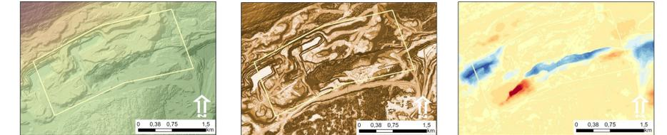
Fig. 8. Left to right: 1m DEM (2019), slope (1st derivative), DoD (2011-2019)
