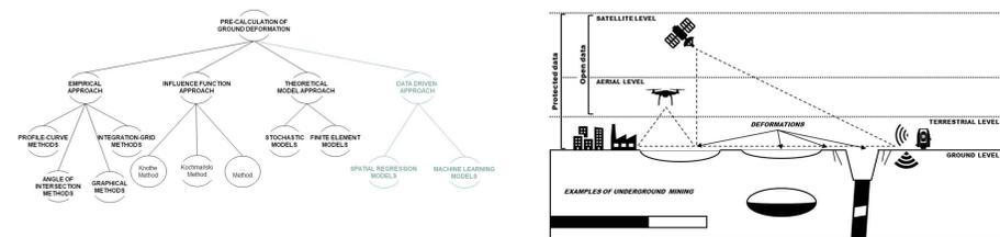
Fig. 1. Classification of approaches used for pre-calculation of mining related ground deformation (based on Kratzsch, 1983; Kwiatek, 1997; modified)
