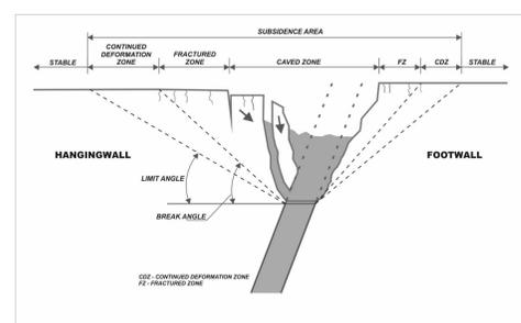
Fig. 3. Rock mass deformation in the sublevel caving (SLC) mining system (Blachowski & Ellefmo, 2012)
