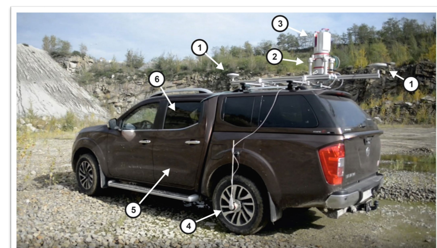
Mobile laser scanning system w trakcie pracy w wyrobisku: (1) GNSS antenna; (2) IMU; (3) Riegl VZ-400i scanner; (4) DMI; (5) power unit (inside the vehicle); (6) driver and control unit – computer with installed software and its operator (inside the vehicle).
