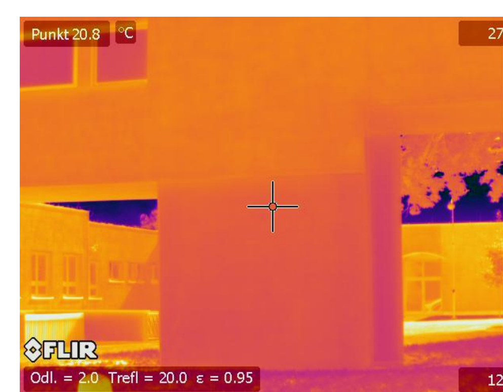
Fig. 7. Temperature distribution outside connector No. 1
