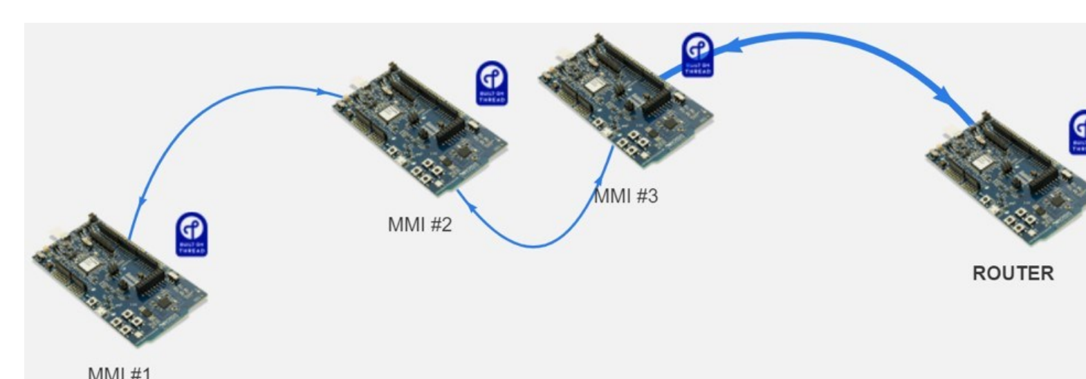
Fig. 6. Sensors connected in series - they transfer data to the router as part of their operation in their range circles. Each sensor provides a transport bridge for the next one on a line. It makes the effective range of all networks much extended within the use of only one gateway
